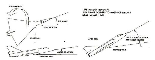
We spoke earlier of control losses which specifically occurred during rudder reversals, but they have also occurred during normal high angle of attack rudder maneuvering. If the aircraft is rolled fast
