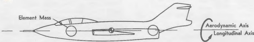
Here the nose/tail masses and CG are aligned with both axes, therefore inertial forces are slight.
